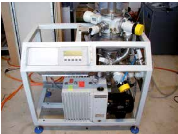
Fully automatic diffusion pump set including controller PCA700D
